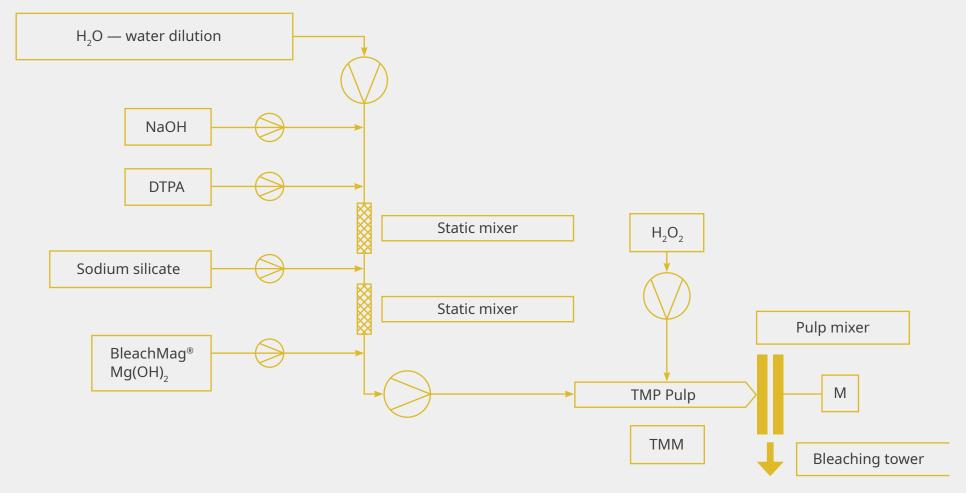
*Pic. 1. Dosing scheme for BleachMag<sup>®</sup> into TMM pulp bleaching process*
